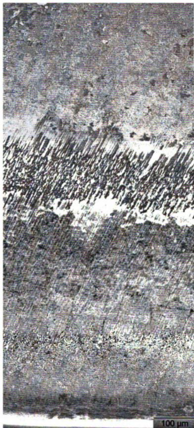
Figure A.1 SEM merged images of crater wear for the corner with 300s machining time
