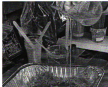
(e) Wetting of fibers with resin
