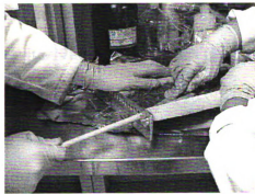
(g) Inserting rods into plate mold
