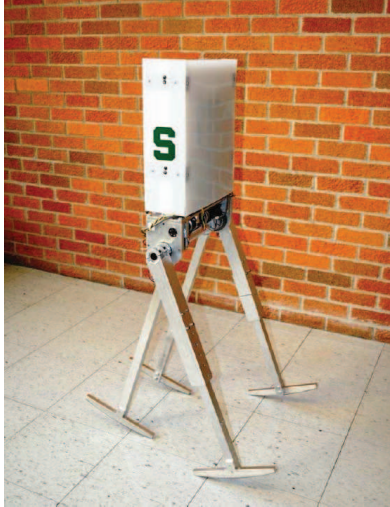
Figure 1.1: Synthetic Wheel Biped (SWB) by Flynn [1]
