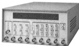
Figure 18: Stanford Research Systems delay box.
