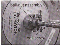
Figure 4.4. Assembly of the ball-screw mechanism and motor
