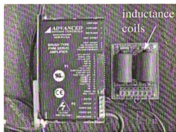
Figure 4.15. Advanced motion servo power amplifier with inductance coil
