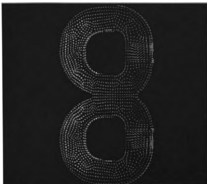
Figure 9.10 Absolute velocity vectors representing flow around the core in the channel
