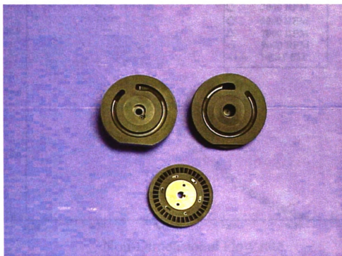
Figure 7.6 Impeller with both side channels
