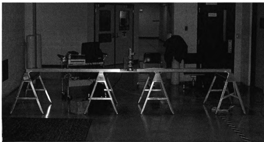
Figure 4.26: The SAR VI depends on the user to manually move the radar down a metal track.
