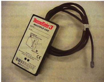
Figure 3-12: Time Temperature Indicator (Sensitech Inc.)
