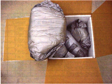
Figure 3-14 Setup of Packages for Vibration and Drop Test.
