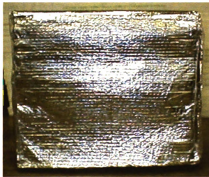
Figure 1-7 Insulated pallet blanket
