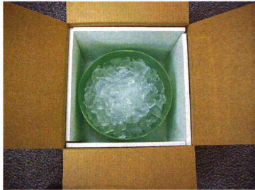
Figure 3-13 Experimental setup of R-value measurement.
