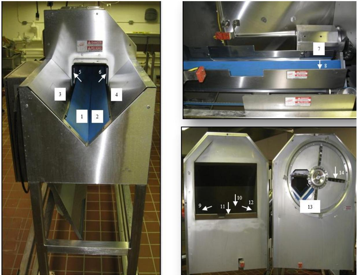
Figure 2.1: Sampling locations on the shredder. Locations with number of 1,3,5,7,9,11, and 13 were sampled before 90.7 kg of iceberg lettuce was processed. Locations with number 2, 4, 6, 8, 10, 12, and 14 were sampled after 90.7 kg of iceberg lettuce was processed
