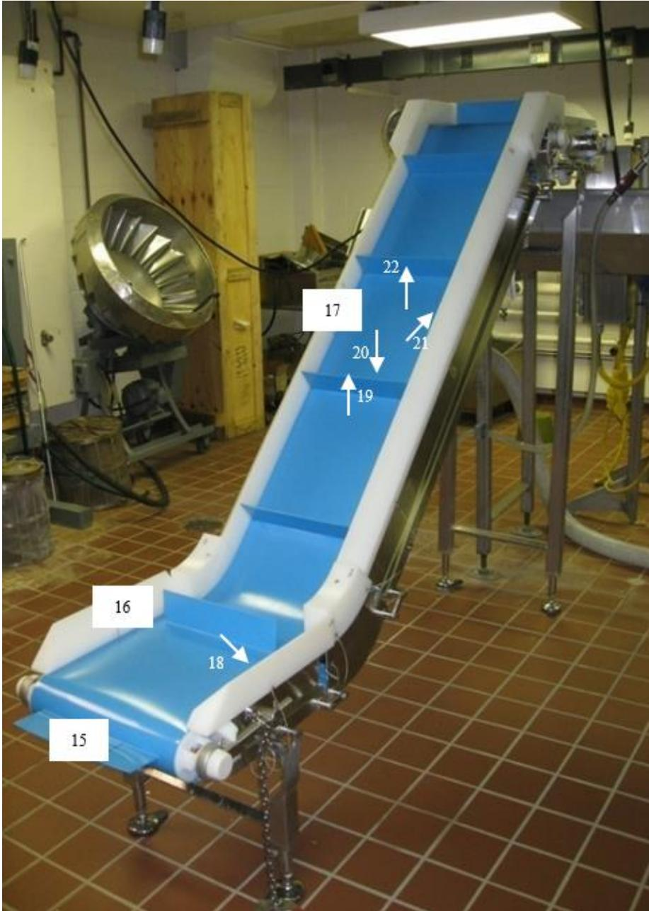
Figure 2.2: Sampling locations on the conveyor. All sampling locations were sampled after 90.7 kg of iceberg lettuce was processed when the shredder was contaminated. While the conveyor was contaminated, locations with number of 15, 17, 19, and 21 were sampled before 90.7 kg of iceberg lettuce was processed. Locations with number 16, 18, 20 and 22 were sampled after 90.7 kg of iceberg lettuce was processed.
