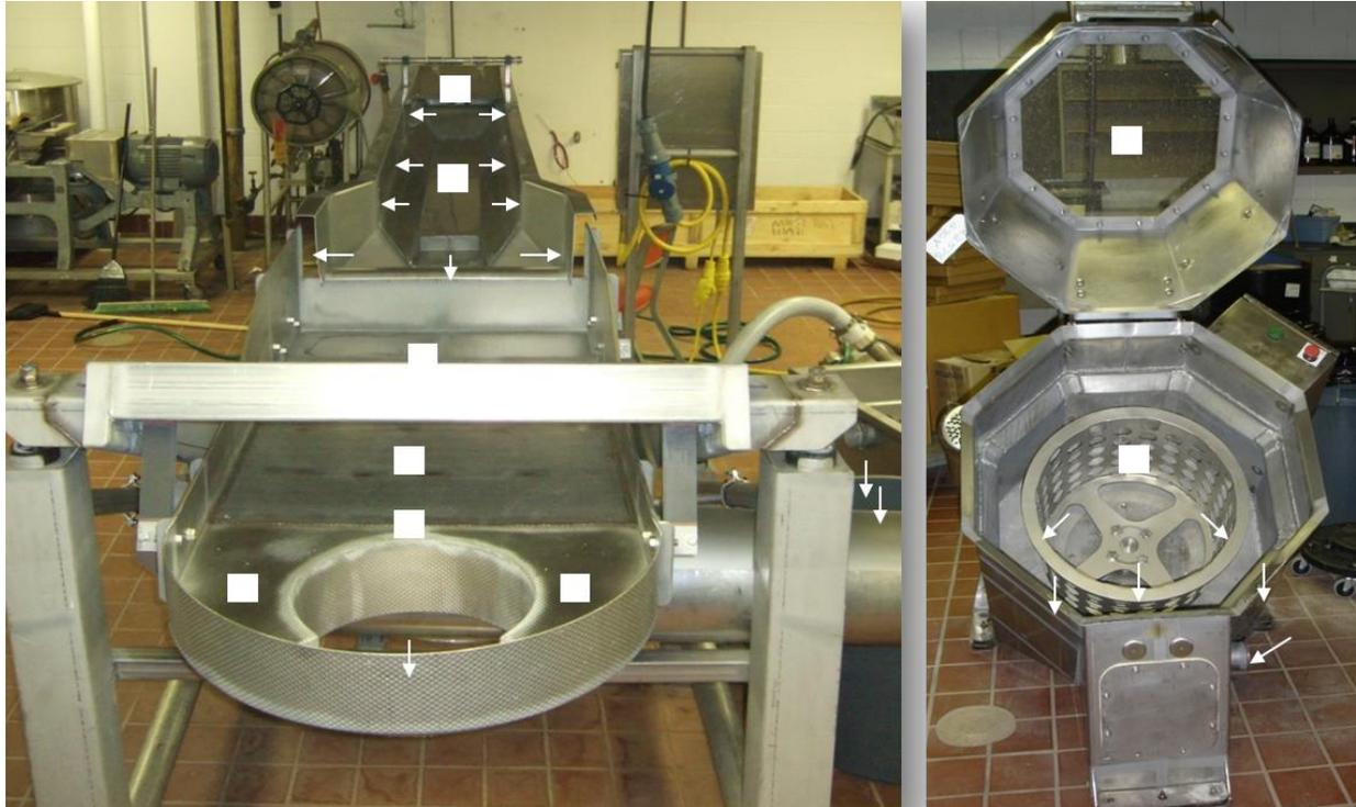
Figure 2.3: Sampling locations on the flume tank, shaker table and centrifugal dryer.
