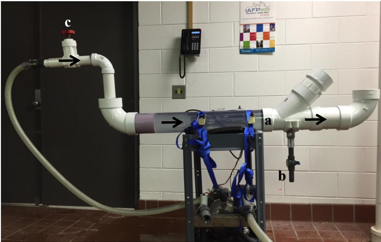
Figure 3.1: Custom-made pipe system. Point 'a' is the inoculation port in the water study and the lettuce insertion port in the lettuce study. Point 'b' is the water sample spout. Valve 'c' is an eye valve for controlling water flow rates.
