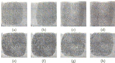
Figure 2.15: Eight 300 \times 300 fingerprint impressions acquired using the Veridicom sensor. Images (a) - (d) correspond to the right index finger of one subject, and images (e) - (h) correspond to the right middle finger of another subject. The images were resized to 256 \times 256 to speed-up Fourier operations.
