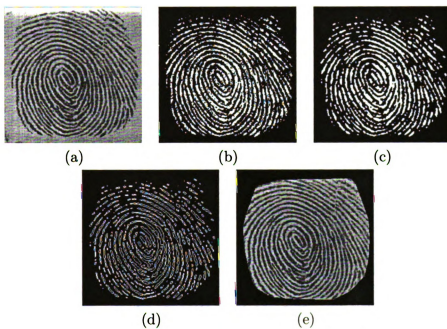
Figure 2.8: Segmenting a fingerprint image. (a) The original fingerprint image. (b) The binarized fingerprint image. (c) The median filtered image. (d) The edge image outlining the ridges. (e) The segmented fingerprint image.
