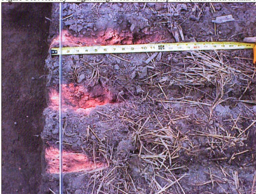
Figure C13: Aerway™ light tillage void cavities, top view (excavation normal to travel)
