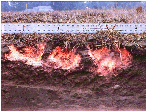
Figure C15: Aerway™ aggressive tillage void cavities, side view (excavation normal to travel)
