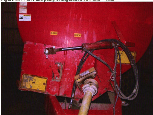
Figure C8: Valve and pump configuration on Nuhn™ tank
