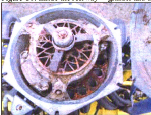
Figure C6: Inside the Aerway™ grinder and distribution manifold
