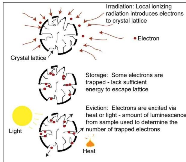
**Figure 2.8: Illustration of the methods used to obtain a luminescence date (modified from Aitken, 1998).**
