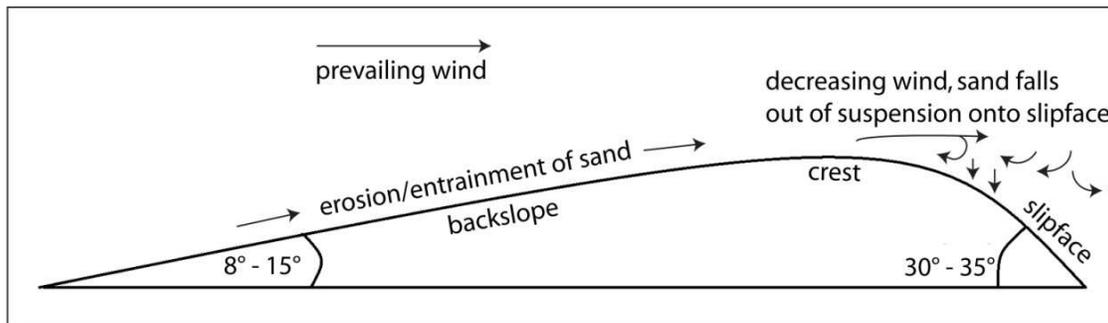
**Figure 2.2: Cross-section of a typical sand dune (modified from Ritter, 1986).**
