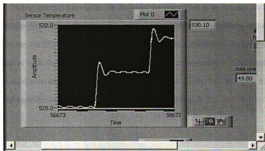
Figure 4. 30 The transition between temperatures during the temperature dependent measurement.
