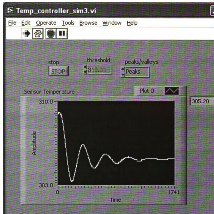
Figure 4. 18 A snapshot of LabVIEW display on the system temperature with P, I, D = 50, 0, 0
