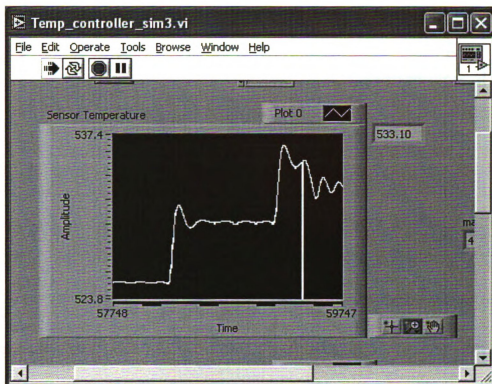
Figure 4. 32 Reset the PID values to 100, 0, 0. The white vertical line indicated when the PID was changed.
