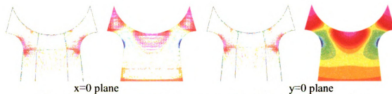
Fig. 5.2 3-D flow pattern (e) at pressure ratio of 0.9 and 23.1% opening
