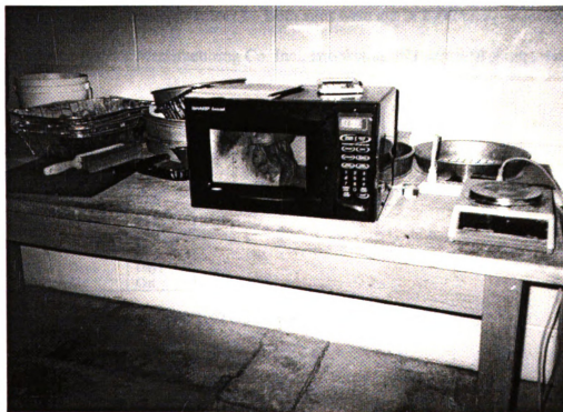
Fig 2. Microwave oven and scale to determine the moisture level.
