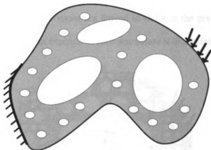
Figure 4.3: A typical structure with macro-scale heterogeneities (perforations)
