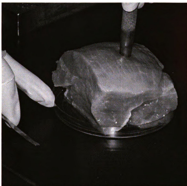
Figure 19. Coring turkey breast with the Warner-Bratzler hand-coring device.
