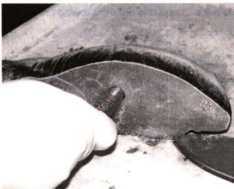
Figure 13. Sampling split turkey breast with the Warner-Bratzler hand coring device
