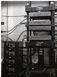
Figure 3.2 Carver Laboratory Press used for compression molding
