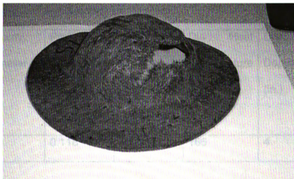
Figure 5.4 Kenaf-PP/MAPP composite formed in ambient conditions
