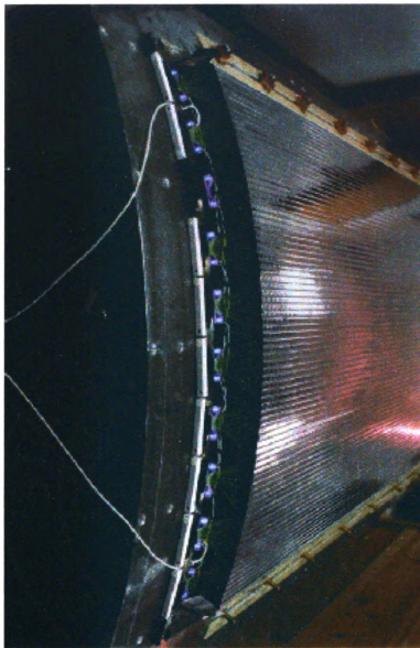
Figure 2.14: A portion of the DØ central preshower detector, a thin cylindrical detector mainly consisting of scintillating fibers.
