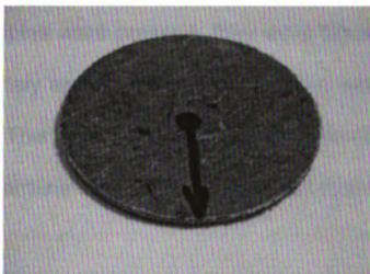
Figure 8. Squeeze flow test sample before testing.
