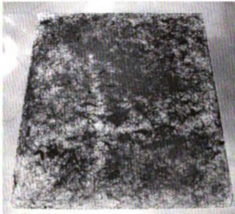
Figure 4. Chopped Kenaf fibers sandwiched between two PP sheets.
