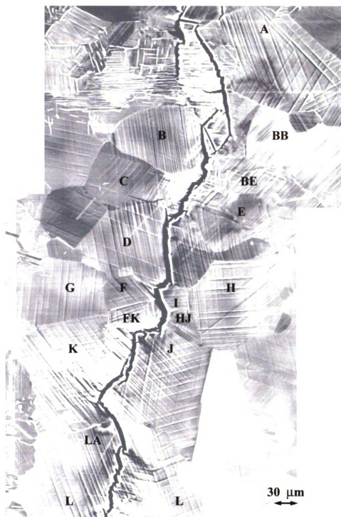
Figure 4.18. Composite BSE image of the crack with the notch on the top and the crack tip located towards the bottom of the image. The grains that are close to the crack path are labeled as shown.
