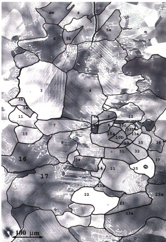
Figure 6.1. The undamaged microstructure below the primary crack was analyzed for grain orientations, and the grains were labeled numerically.
