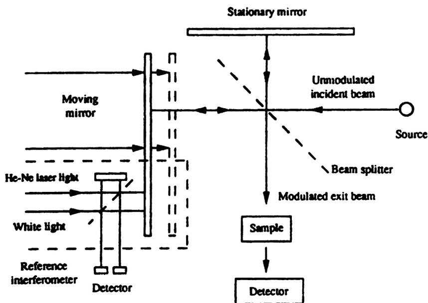
**Figure 3:** Schematic of a Michelson interferometer.
