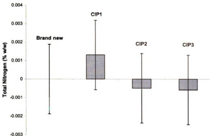
**Figure 13:** Total nitrogen contents (% w/w) of a brand new filter bag and three CIP cleaned Group 3 filter bags. CIP1, CIP2, and CIP3 are Group 3 filter bags.
