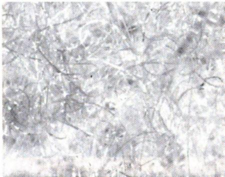
**Figure 7:** Simatek brand new, unused filter bag, clean air side. 30X.
