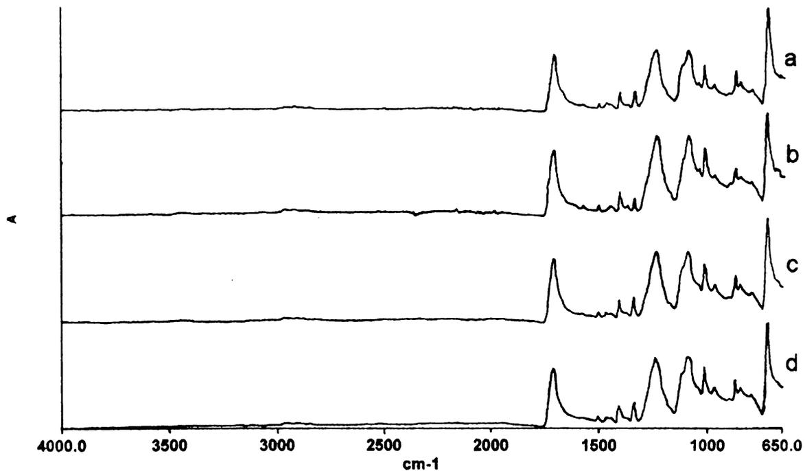
**Figure 10:** FTIR-ATR spectra. (a) Simatek brand new filter bag, clean air side; (b) Simatek brand new filter bag, product side; (c) Intensiv brand new filter bag, clean air side; (d) Intensiv brand new filter bag, product side.
