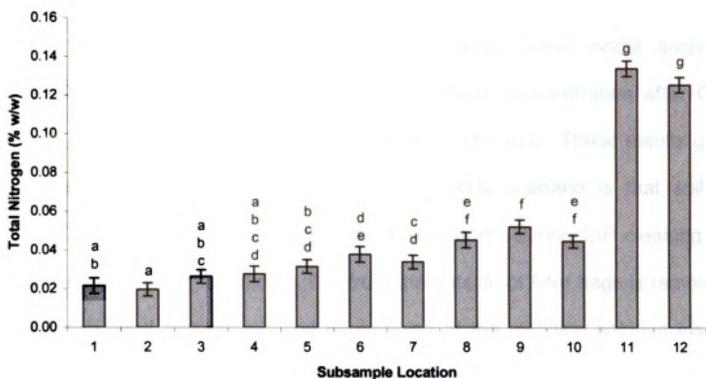
**Figure 14:** Total nitrogen in 6 Group 2 filter bags by sub-sample location. Letters indicate significant differences between locations ( $p < 0.05$ ) by t-test.
