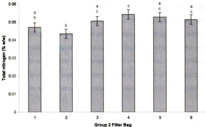
**Figure 15:** Total nitrogen in 6 Group 2 filter bags by filter bag. Letters indicate significant differences between filter bags ( $p < 0.05$ ) by t-test.
