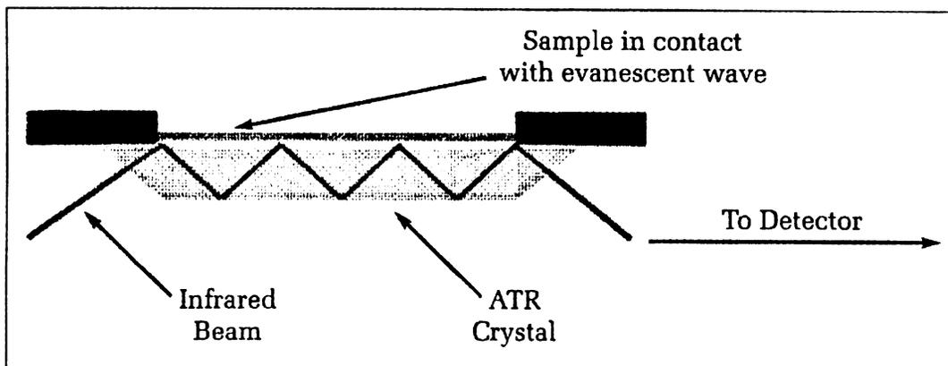
**Figure 4:** An attenuated total reflectance (ATR) sampling accessory.
