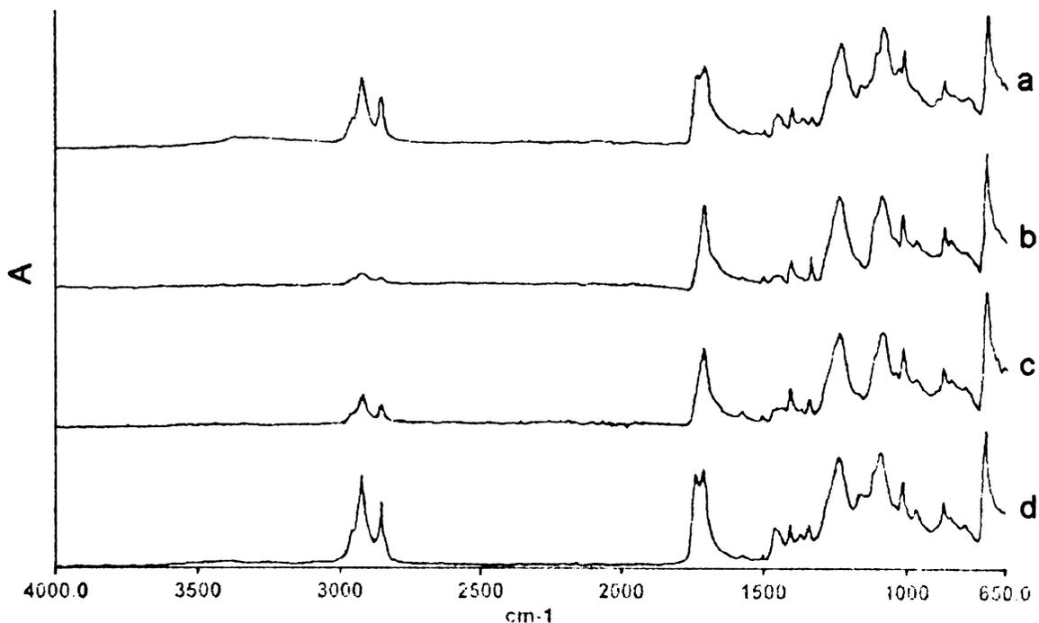
**Figure 12:** FTIR-ATR spectra. (a) Simatek Group 1 used uncleaned bag, product side, sub-sample 5; (b) Simatek Group 1 used uncleaned bag, clean air side, sub-sample 5; (c) Simatek Group 1 used CIPed bag, product side, sub-sample 2; (d) Simatek Group 1 used CIPed bag, product side, sub-sample 5.
