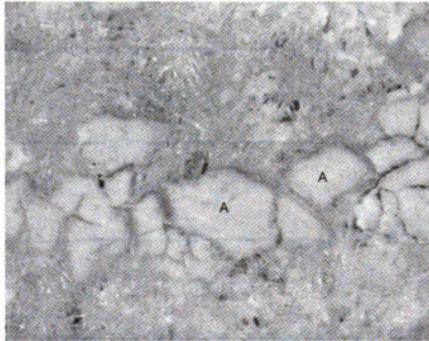
**Figure 9:** Intensiv-Filter Group 2 filter bag, product side along side wall of filter bag at a location showing visible powder residue (A). 20X
