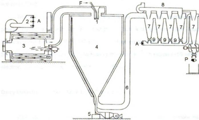
**Figure 1:** Vertical spray dryer with indirect air heater and powder recovery cyclones. (1) Atomizer, (2) Fan with air filter, (3) air heater, (4) spray drying chamber, (5) power source for pneumatic collector, (6) discharging pipeline for powder and air, (7) cyclone separators system, (8) air discharging pipeline, (9) valve. F, feed; A, air; P, product.
