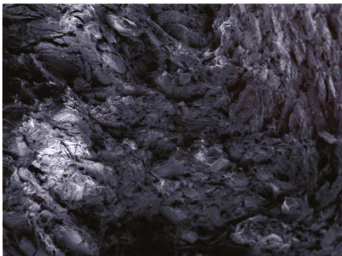
A control 100 phr pine-PVC composite at 50x.
