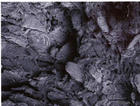
A 100 phr pine-PVC composite after 5 WFT cycles at 25x.
