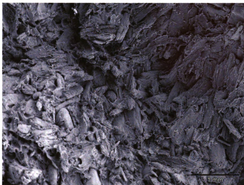
15 FT only maple-HDPE composite at 25x resolution (cont'd).
