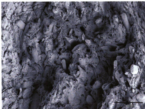
A 100 phr pine-PVC composite after 5 WFT cycles at 25x.
