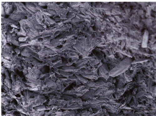
Control maple-HDPE composites at 25x resolution.
