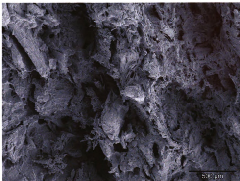
100 phr pine-PVC composites after 5 FT only cycles at 50x (cont'd).
