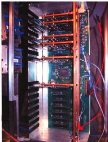
Figure 4.27: Image of a motherboard inside its shielding box. Also shown are the cooling bar configuration designed to keep the ASICs cool in vacuum.
