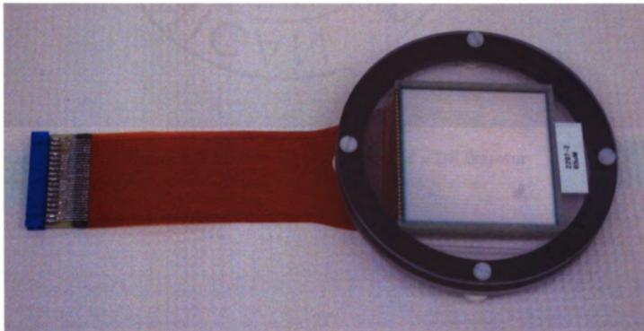
Figure 4.7: Picture of the front side of a DE detector
