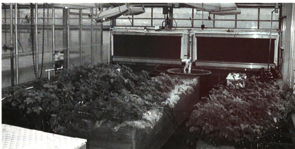
Figure 2-1. Compartmentalized boxes lined with plastic sheeting. Each box contains individual water content reflectometers and irrigation outlets.
