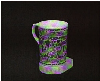
Rec. Image 6 using VM5b (PSNR = 32.10 dB, bit rate = 0.9991 bpp)
