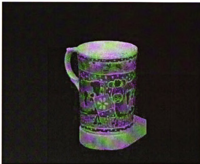
Rec. Image 6 using VM5b (PSNR = 27.42 dB, bit rate = 0.8163 bpp)
