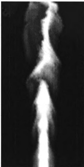
Figure 3.10: Contours of mixture fraction from the particles for case 4 (1-g , flamelet). The domain shown is 0 < x/D < 20 , y = 0 , -5 < z/D < 5 .
