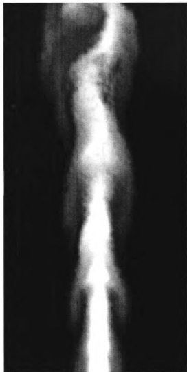
Figure 3.8: Contours of mixture fraction from the particles for case 3 (1-g , 1-step). The domain shown is 0 < x/D < 20, y = 0, -5 < z/D < 5 .
