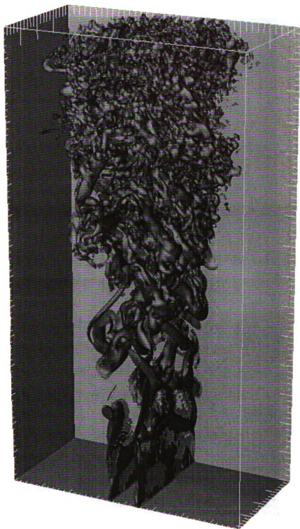
Figure 1.2: Iso-surfaces of vorticity in the 3-D nonreacting jet at the final time of the simulation, t/t_0 = 4 . The domain shown is 1 < x/h < 16 , -4 < y/h < 4 , 0 < z/h < 4 .
