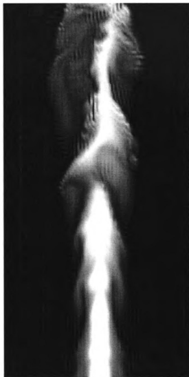
Figure 3.9: Contours of mixture fraction from the finite difference solution for case 4 (1-g , flamelet). The domain shown is 0 < x/D < 20, y = 0, -5 < z/D < 5 .
