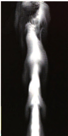
Figure 3.7: Contours of mixture fraction from the finite difference solution for case 3 (1-g , 1-step). The domain shown is 0 < x/D < 20, y = 0, -5 < z/D < 5 .
