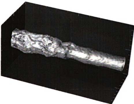
Figure 2.8: Isosurface of \langle T \rangle_L = 1500K from the flamelet flame D case. The domain shown is 0 < x/d < 20 , -5 < y/d < 5 , -5 < z/d < 5 .
