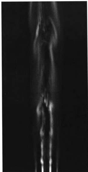
Figure 3.4: Contours of vorticity magnitude (0-10) for case 1 (0-g , 1-step). The domain shown is 0 < x/D < 20, y = 0, -5 < z/D < 5 .
