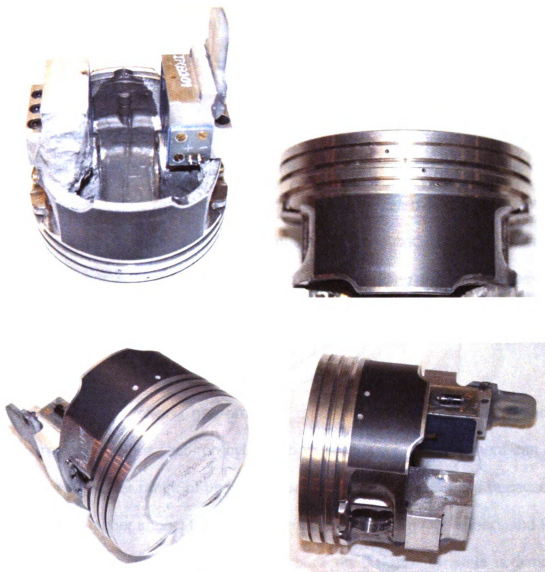
FIGURE 70. Piston equipped with IR telemetrics
