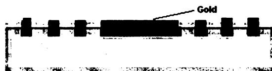
Figure 6.23 After Glass Part Step10: Electroplating: deposition of 4 microns gold(Au)
