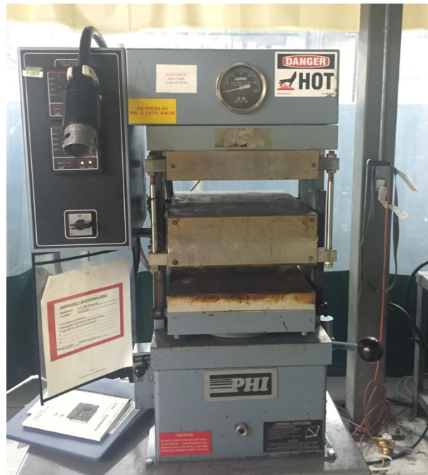
Figure 4-7: PHI press used in molding nylon based panels
