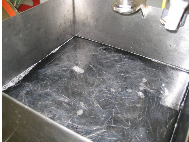
Figure 4-4: Thermoplastic and carbon fibers mixed with white water in deckle box
