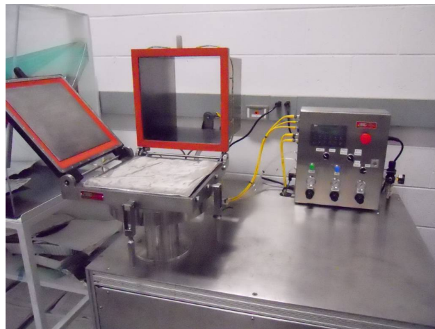
Figure 4-3: Formax sheet former. Shown with deckle box and couching plate rotated up
