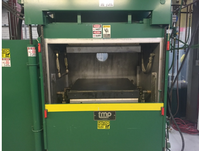
Figure 4-8: TMP press used for molding PEEK based panels
