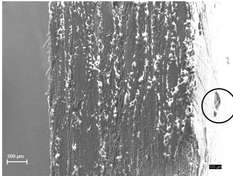
Figure 6-6: Photomicrograph of panel 012 coupon 06 (Nylon). Surface pit circled in black.
