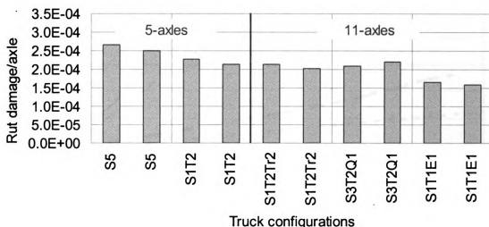
Figure 5-16 Relationship between total number of truck axles, maximum axle group, and truck factor (two replications each)
