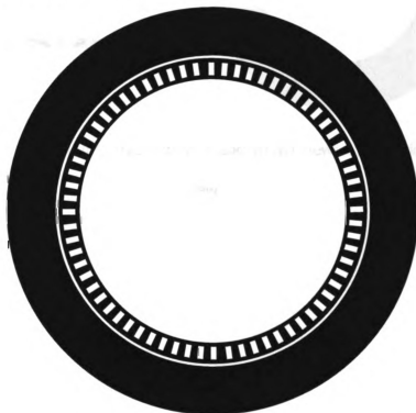
Figure VIII.4: Positive mask used in step 5 of axial wave rotor fabrication.
