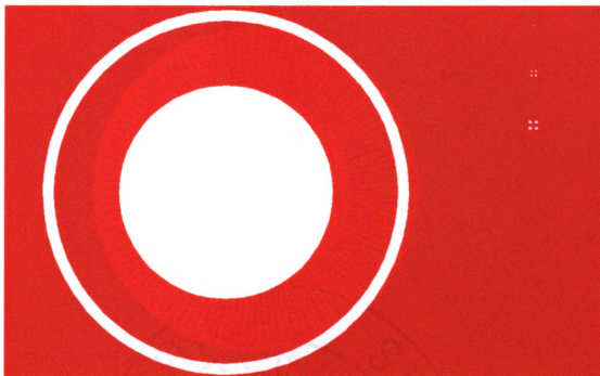
Figure A.7: Mask used for first etch step of rotor wafer 1.
