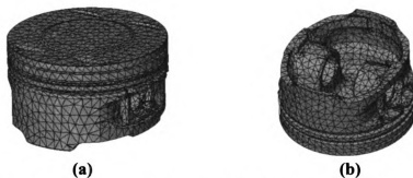
Figure 4.1: Full piston model mesh in COSMOSDesignSTAR, (a) top side, (b) underside
