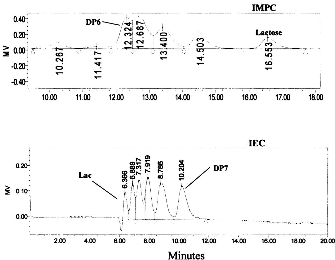
**Figure 4.7. Chromatograms of sugar solutions containing 0.02 mM of lactose and malto-oligosaccharides run with HPLC-grade water at 0.4mL/min for ion moderated partition and ion exclusion chromatography.**
