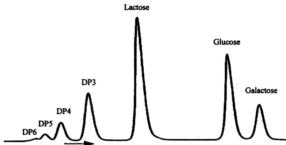
**Figure A.3.1. A typical HPLC chromatogram showing various sugars found in lactose hydrolysis. Elution time (min): 10.1 for DP6, 12.2 for DP5, 12.8 for DP4, 13.8 for DP3, 16.2 for lactose, 19.5 for glucose and 20.5 for galactose.**
