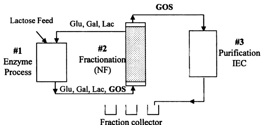
**Figure 1 - Schematic of the overall GOS manufacture process. Objectives or phases are labeled as #1, #2, and #3.**
