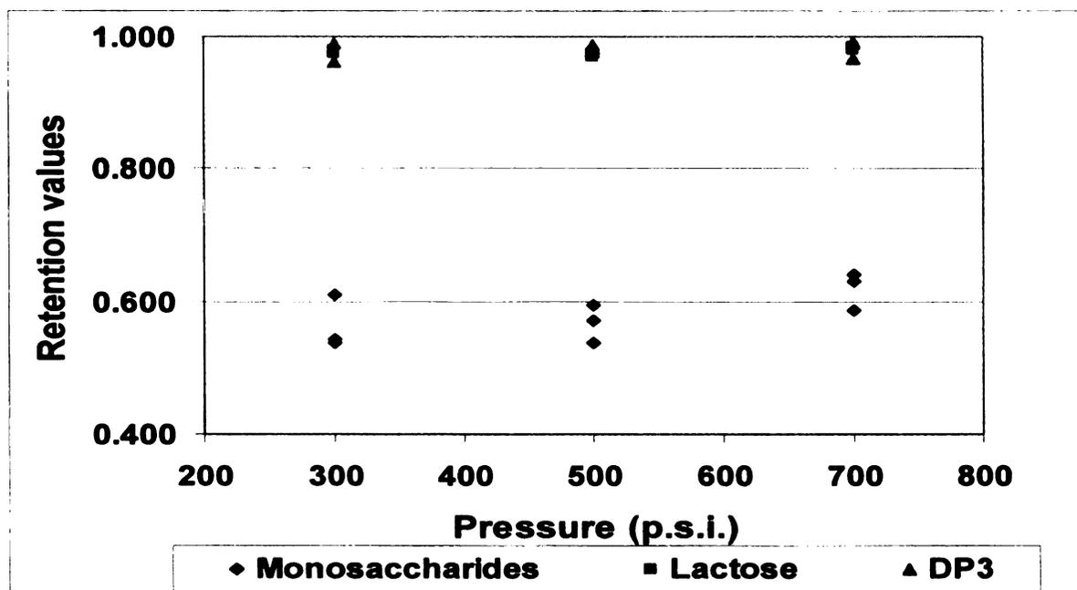
Figure 3.3 - Retention values of sugars in a nanofiltration system at various pressures at 50°C.
