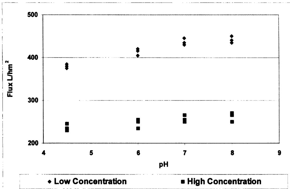
**Figure 3.5. The effect of pH on flux of high and low concentrated oligosaccharide mixtures in NF.**
