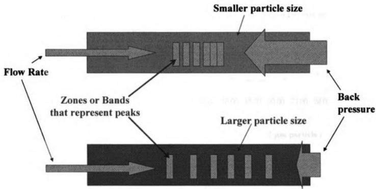
**Figure 4.3. Illustration of backpressure effect on peak co-elutions within small and large particle size resins in HPLC columns.**
