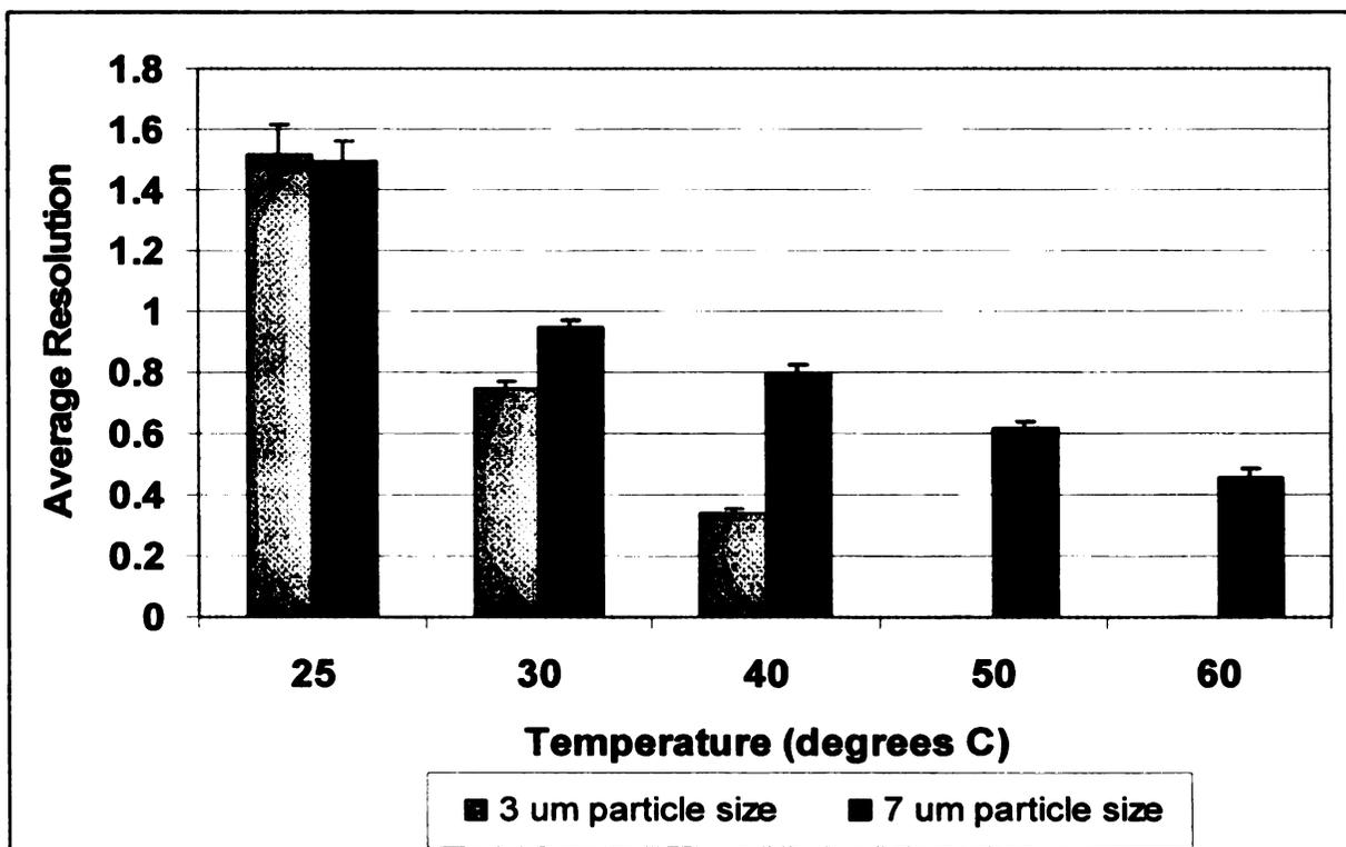
**Figure 4.5. Temperature effect on average resolution for 3 and 7  $\mu\text{m}$  particle size resin.**
