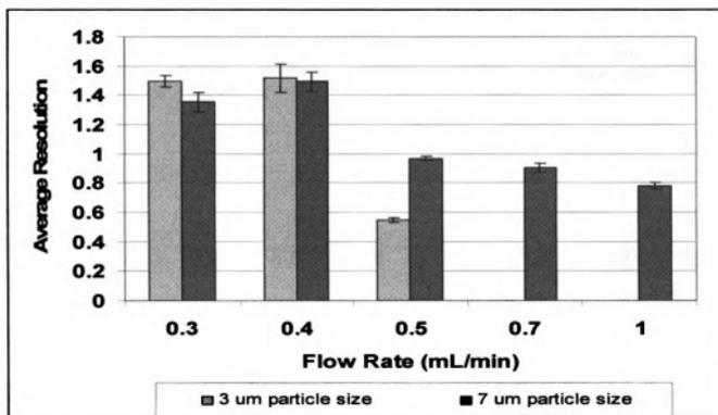
**Figure 4.1. Average resolution for anion exclusion chromatography of 3- and 7- $\mu$ m particle size at various mobile phase (HPLC grade water) flow rates.**
