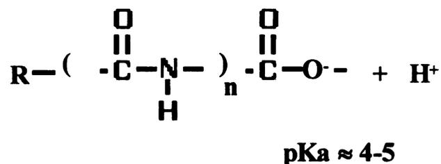
**Figure 3.6. Structure of polyamide polymer with carboxylic acid end group.**
