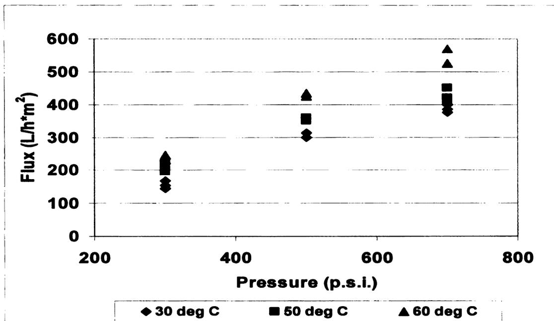
**Figure 3.2 - Flux of sugar solution at various pressures and temperatures.**
