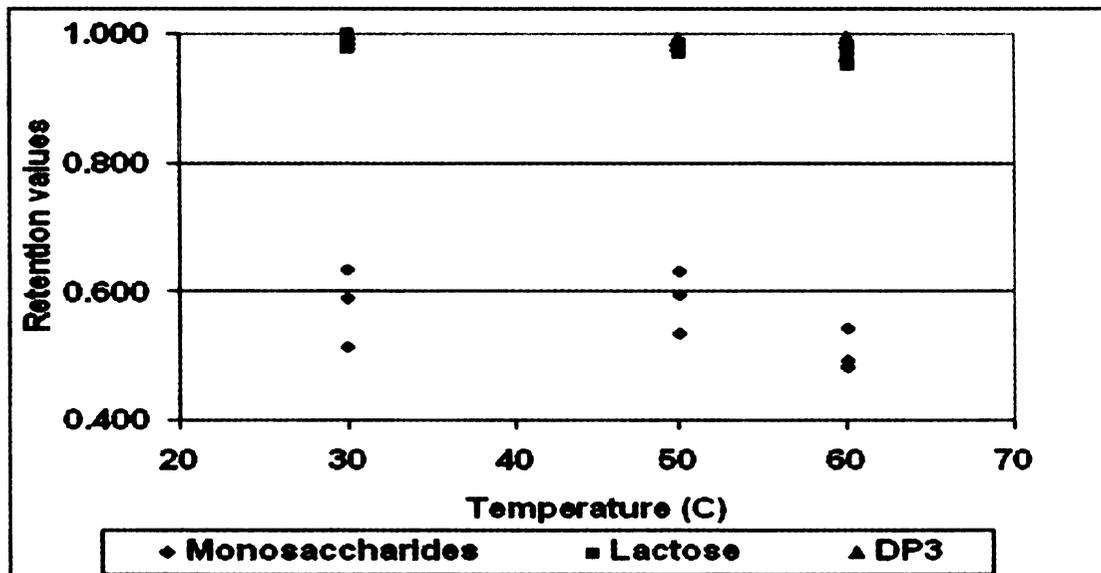
Figure 3.1 - Retention values of sugars in a nanofiltration system at various temperatures at 500 p.s.i.
