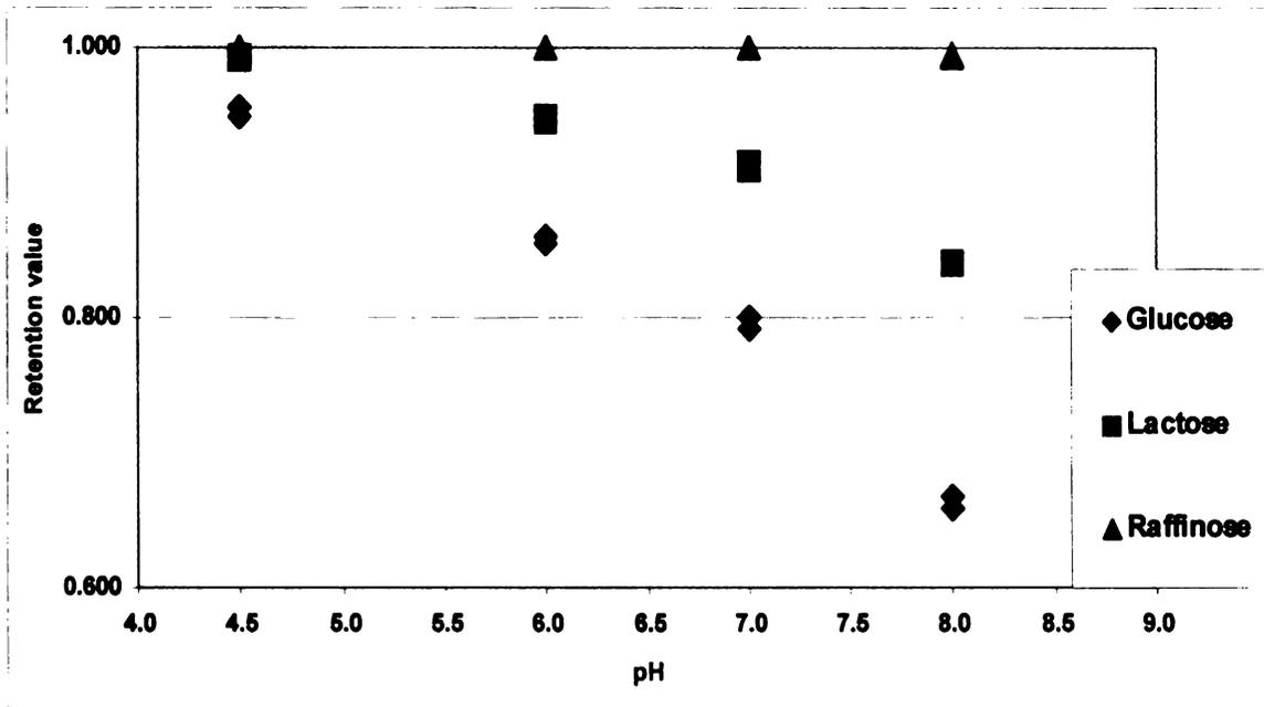
**Figure 3.4. Effect of pH on retention values of model solutions containing ~7mM of glucose, lactose and raffinose.**
