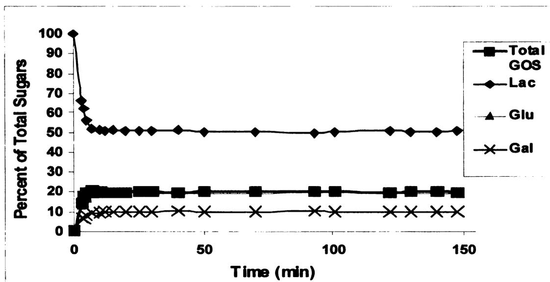
**Figure 2.5 - Percent of total sugars over time within an immobilized-enzyme system with constant feed of 27% (w/v) lactose. Each datum represents the mean of three replicates with CV% from 0.20 to 5.3%.**
