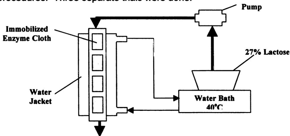
**Figure 2.2 - Single-pass immobilized enzyme system with continuous 27% (w/v) lactose feed at 40°C, pH 4.5 and optimum flow rate.**
