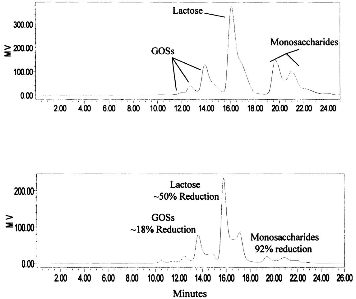
**Figure A.6.1. HPLC chromatograms of various sugars present during initial (top) and post-diafiltration (bottom) samples.**
