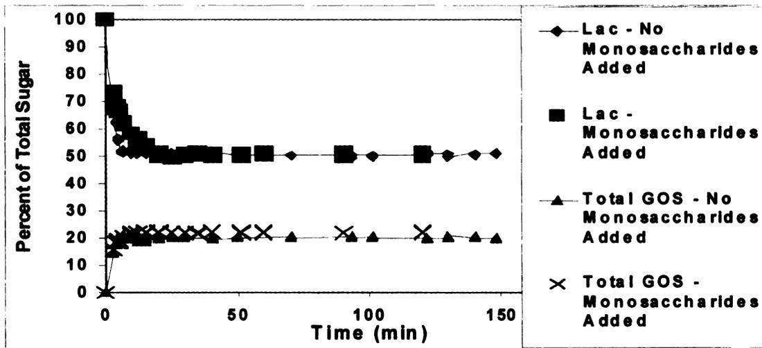
Figure 2.7 - Lactose and total GOS percent over time during continuous immobilized-enzyme system where 27% (w/v) lactose feed either contained no monosaccharides or 0.87% (w/v) glucose and 0.43% (w/v) galactose. Each datum represents the mean of three trials (CV% from 0.21 to 3.9%).
