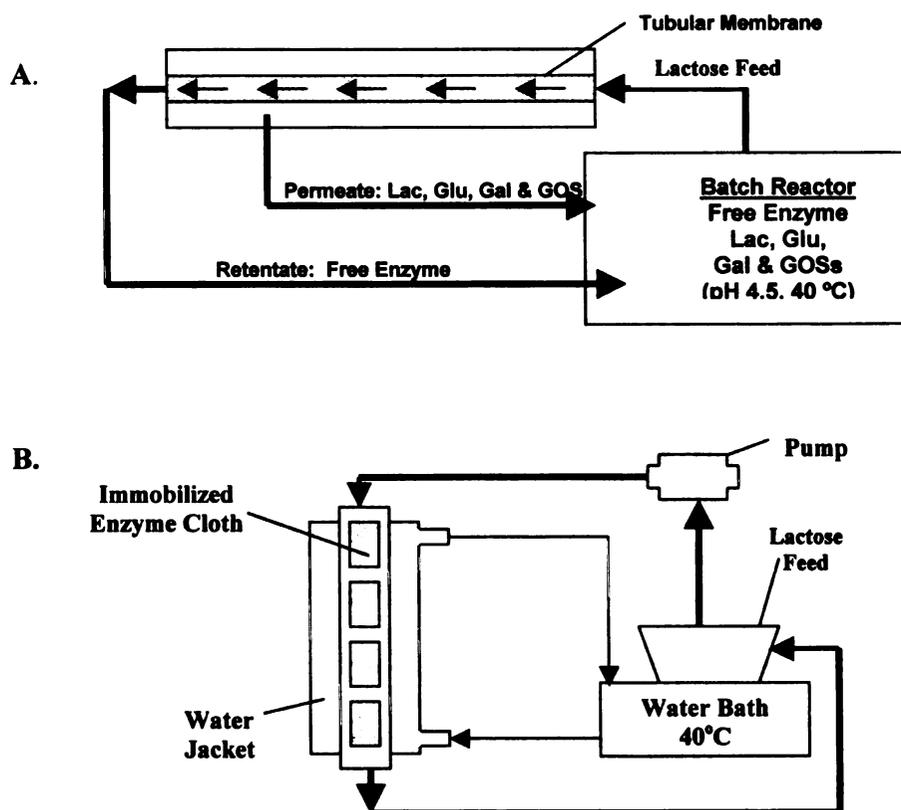
**Figure 1.1 - A) A recycled UF membrane free-enzyme system that contains optimum initial  $\beta$ -galactosidase and lactose concentrations at pH 4.5, 40 °C; B) A recycled immobilized-enzyme system, which uses optimum immobilized cloth amount and initial lactose concentration at pH 4.5, 40°C.**
