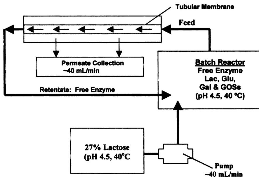
**Figure 2.1 - Continuous free-enzyme system using UF membrane filtration to separate sugars from enzyme with 27% (w/v) lactose feed at pH 4.5 and 40°C.**
