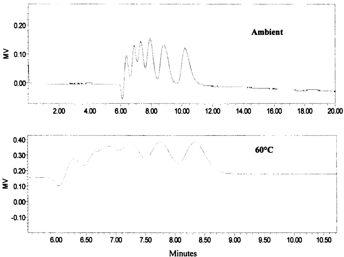
**Figure 4.6. HPLC chromatograms of 0.02 mM sugar mixture (lactose and malto-oligosaccharides (DP3-7)) at ambient and 60°C column temperature, with 7 $\mu$ m particle size resin and 0.4 mL/min flow rate of HPLC-grade water.**
