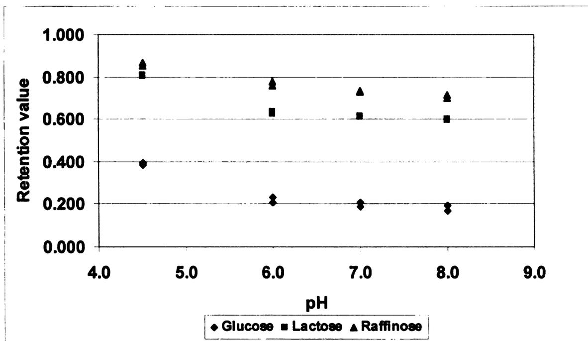
**Figure 3.7. Effect of pH on retention values of model solutions containing ~200, 330 and 66 mM of glucose, lactose and raffinose, respectively.**
