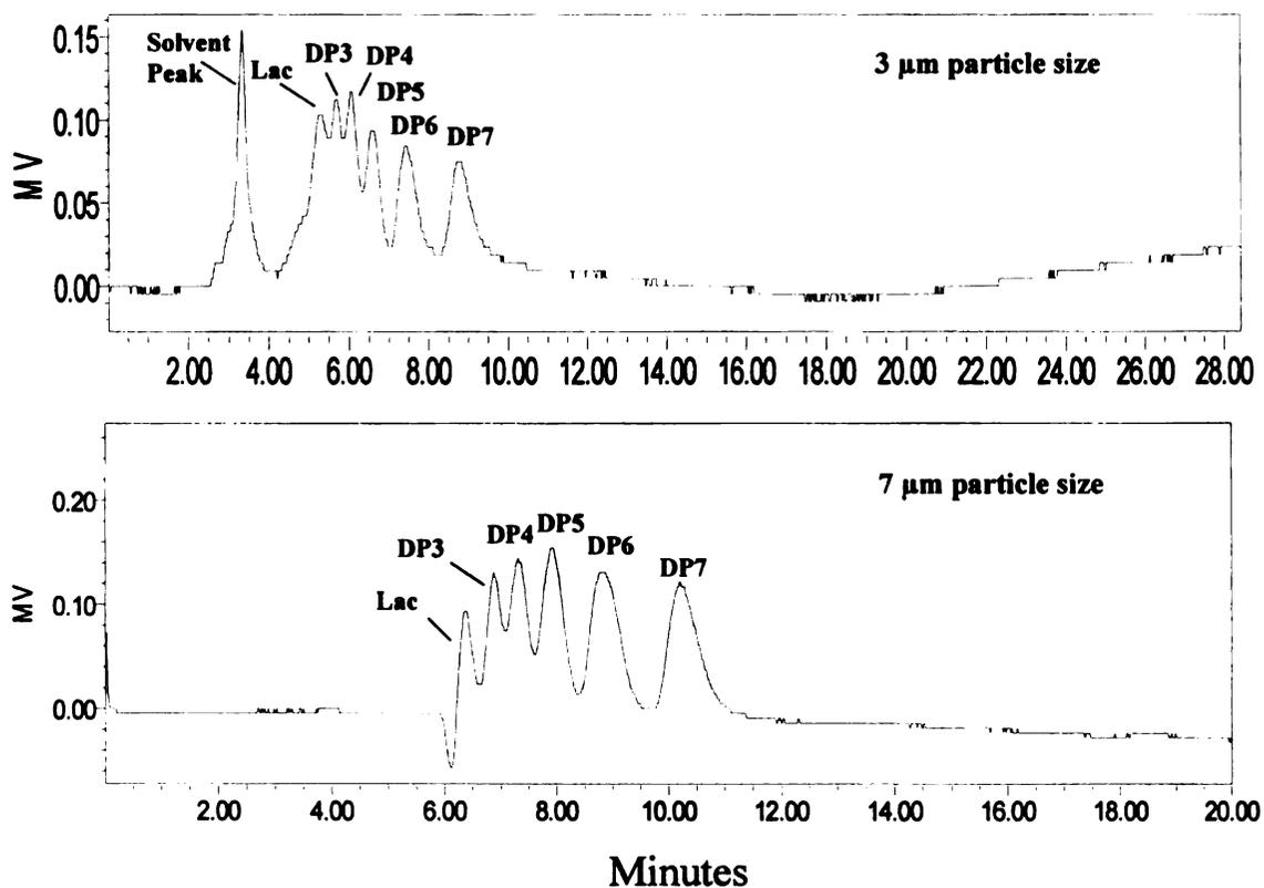
**Figure 4.4. HPLC chromatograms of 0.02mM sugar mixture of lactose and malto-oligosaccharides (DP3-7) at ambient column temperature, HPLC-grade water mobile phase and 3 (top) and 7 (bottom) µm particle size resin.**
