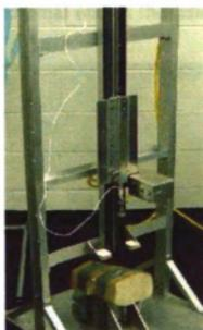
**Figure 5.** The gravity-driven impact fixture. The impact chair was situated under the fixture with the animal's femur vertical and the patella directly under the impact sled. Note the impact sled stopped at one of the electronic braking fixtures that prevented multiple
