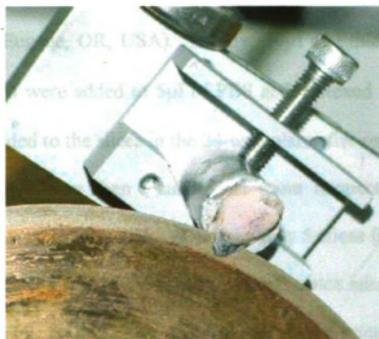
**Figure 7.** The excised patellae were cut through their thickness using an Isomet saw as shown in the photo. Patellae were glued to a metal base, and kept moist with PBS during cutting.
