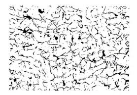
Figure 13. Microstructure of iron R6S, in the interior. Treated with 0.8% strontium. Nital etch. 100X.
