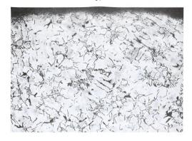
Figure 18. Microstructure of iron R7FS2, at the surface. Treated with 0.4% ferrosilicon. Nital etch. 100X.
