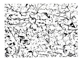
Figure 7. Microstructure of Iron R32C, in the interior.
