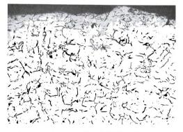
Figure 17. Microstructure of iron R11CS2, at the surface. Treated with 0.8% calcium-silicon. Nital etch. 100X.
