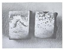
Figure 8. Macrostructures of irons quenched at the start of eutectic solidification. Left picture: Iron R9S2, treated with 0.24% strontium. Right picture: Iron R9X2, untreated. Nital etch. Approximately 1.5X.
