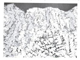
Figure 15. Microstructure of Iron R6B, treated with 1.0% barium. Nital etch. 100X.
