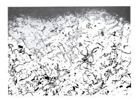
Figure 5. Microstructure of Iron R32C, at the surface. Treated with 0.2% calcium. Nital etch. 100X.
