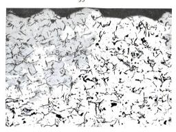
Figure 16. Microstructure of iron R11BS2, at the surface.
