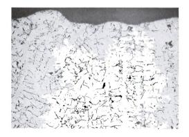
Figure 19. Microstructure of iron R712, at the surface. Treated with 0.4% Inoculoy. Nital etch. 100X.
