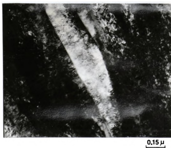
Figure 24. TEM microstructure of martensite obtained by process A with 70% cold rolled.
