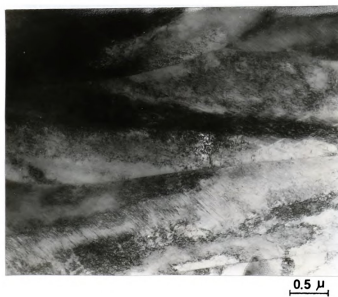
Figure 21. Optical microstructure of as-quenched Fe-30.4%Ni alloy
