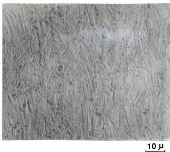
Figure 23. Optical microstructure of martensite obtained by process A 70% cold rolled.
