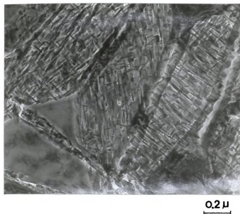
Figure 33. Microstructure of aged Fe-30.4%Ni martensite process A with 70% cold rolling, aged at 335°C, 1000 h.
