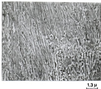
Figure 34. SEM microstructure of aged martensite, process B with 70% cold rolling, aged at 335°C, 1000 h.
