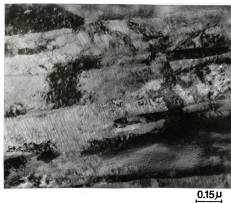
Figure 26. TEM microstructure of martensite obtained by process B with 70% cold rolling.
