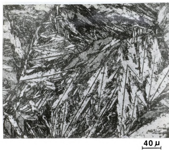
Figure 21. Optical microstructure of as-quenched Fe-30.4%Ni alloy
