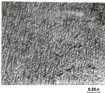
Figure 29. Typical precipitates formed after ageing at 335°C for 1000 hours.
