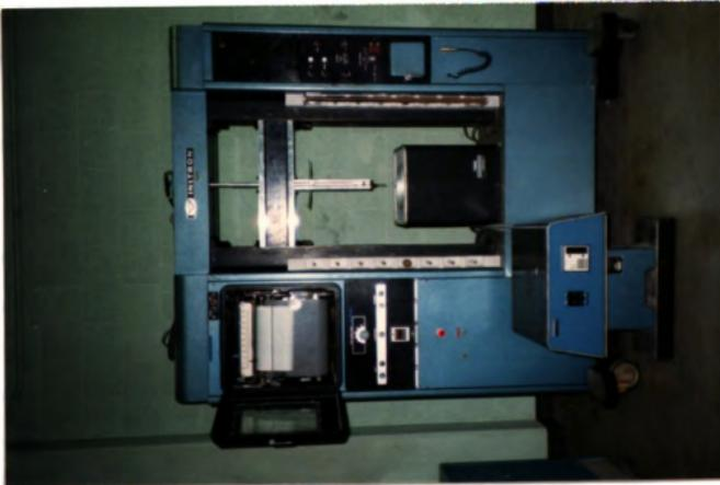
Figure 2. An Apparatus for Three Point Bend Test at Elevated Temperature. A: Universal testing machine. B: Resistance-Heating Furnace. C: Three point bend test fixture.
