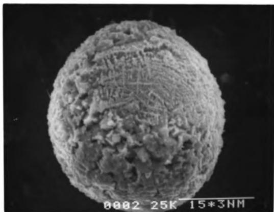
Figure 10. Scanning Electron Micrographs of (A) Magnetic Particle Without Chemical Etching (1500X Magnification), (B) and (C) Magnetic Particle After HF + HCl Etching for 15 Minutes (2000X Magnification)
