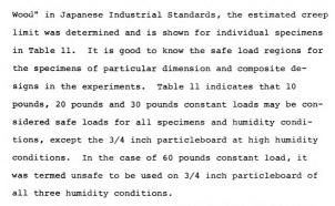
The result shows that the influence of moisture content on the creep limit in bending is not negligible and that the creep limit in bending should be considerably reduced for materials with a high moisture content.
