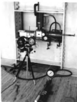
Fig. 6.17.20. Biaxial loading device and photo stress large field meter.
