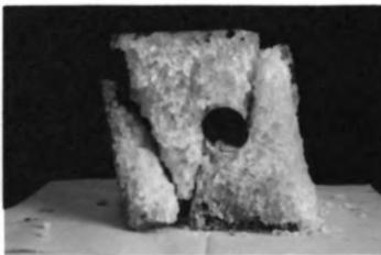
Fig. 6.6.20. Failure of a circular opening under a uniaxial stress of 2,500 psi.
