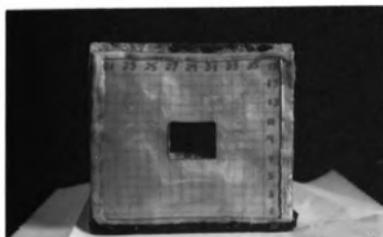
Fig. 6.10.20. Failure of a square opening under a uniaxial stress of 2,850 psi.
