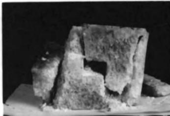
Fig. 6.7.20. Failure of a square opening under a uniaxial stress of 2,750 psi.
