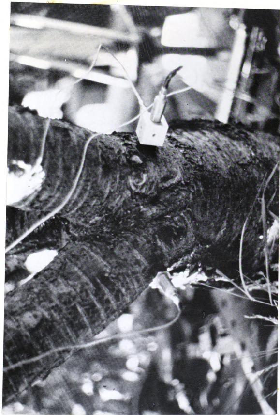
Figure 4.6 Orthogonal location of X and Y accelerometer blocks mounted on a cherry tree trunk.
