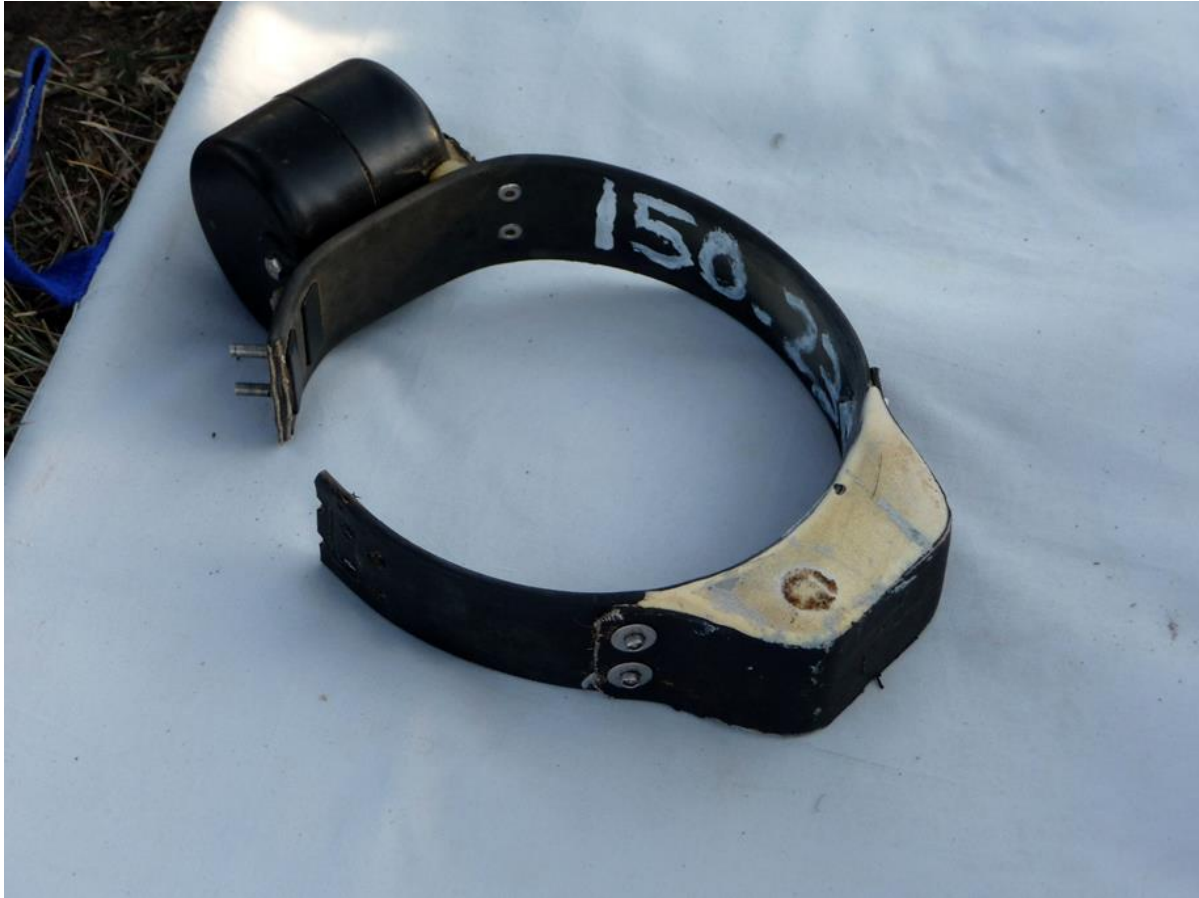
Figure 1.3: A GPS collar like those applied to adult female hyenas in this study.
