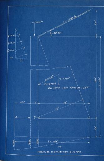
steel than the design required but is put in to bind the base together. The bond stress in the bars near D =  $u = \frac{V b}{0} = \frac{40 \times 6}{1.57} = 153 \text{ pounds per square foot. This value is slightly more than allowable but is used since twice as much steel is used as is necessary.}$
