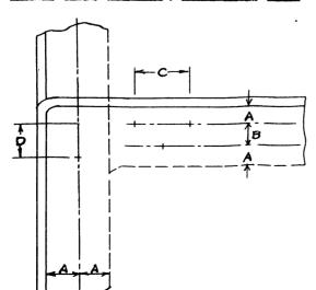
t = 3/8 inches. d = 3/4 " . A = 12 " . B = 1 11/16 " . C = 3 1/16 " . D = 2½ inches . e = 70% Using the diagram on page 432, Creager and Justin, Hydro-Electric Handbook, for the maximum head on the pipe in feet of water, the following results were obtained.
