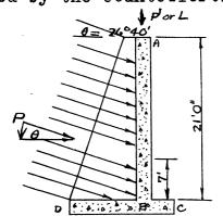
(1) B D is composed of narrow strips uniformly loaded with the dead weight of the slab, the downward weight of the earth, and the upward reaction of the soil.
