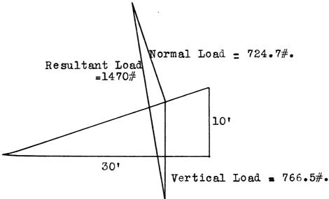
Treating the purlin as a simple beam, supporting a uniform load, the maximum bending moments for the two conditions of loading are:
