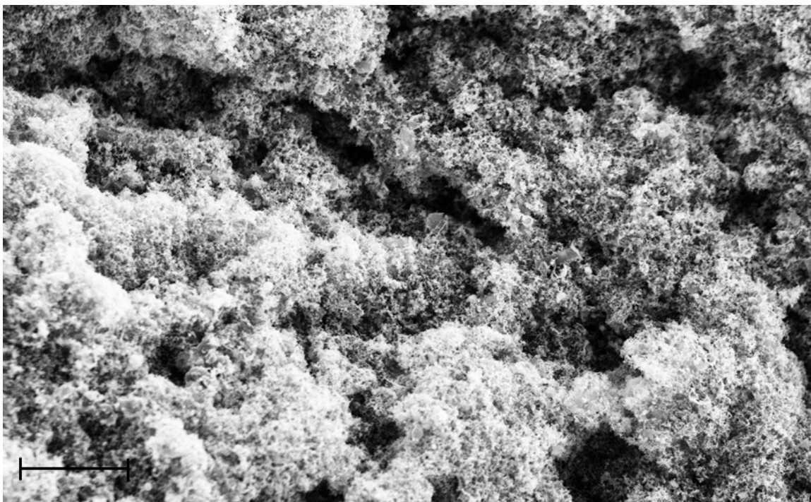
Figure 3-8. SEM image of nylon 6 fibers coated in doped polypyrrole with DI water wash and sonication post-polymerization. Scale bar equal to 100 \mu\text{m} , magnification of 500x, EHT of 30 kV and working distance of 6.0 mm.
