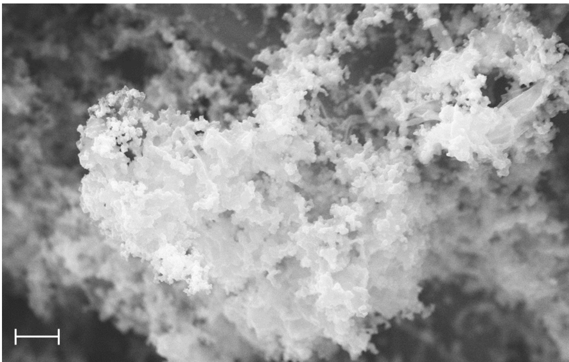
Figure 3-5. SEM image of nylon 6 fibers coated in doped polypyrrole with water as solvent. Scale bar equal to 10 \mu\text{m} , magnification of 2,000x, EHT of 30 kV, and working distance of 8.0 mm.
