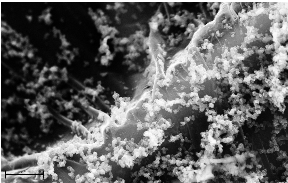
Figure 3-10. SEM image of polypropylene fibers coated in doped polypyrrole. Scale bar at 10 \mu\text{m} , magnification of 5,000x, EHT of 30 kV and working distance of 6.0 mm.
