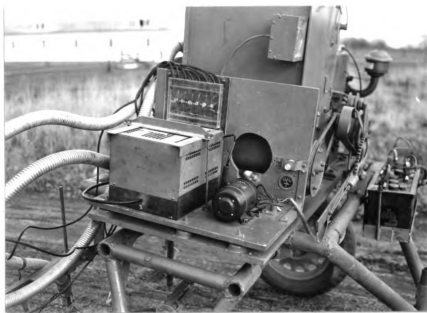
Fig. 10. Side view of experimental duster showing charging equipment.
