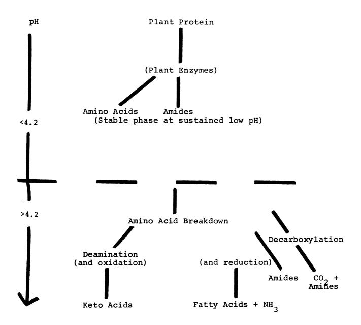
Figure 2. Barnett - Diagram of protein breakdown in silage.
