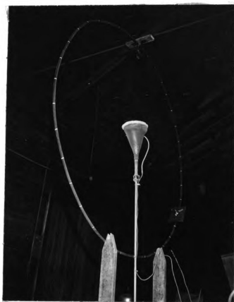
Figure 41. Test stand for determining the radiation pattern of a propane burner
