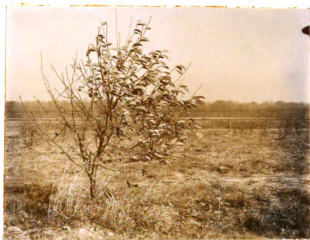
Figure 40. Leaf distribution on a tree 30 feet from a "Frost-guard" three days after test. The leaves remained on the side protected.
