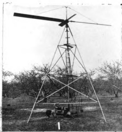
Figure 1. Wind Machine Number One with 15-horsepower gasoline engine
