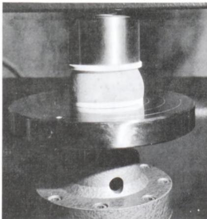
Figure 6.3.--Instron Uniaxial Compression Test with Porous Flat Plate Loading. (Photo 69-83)
