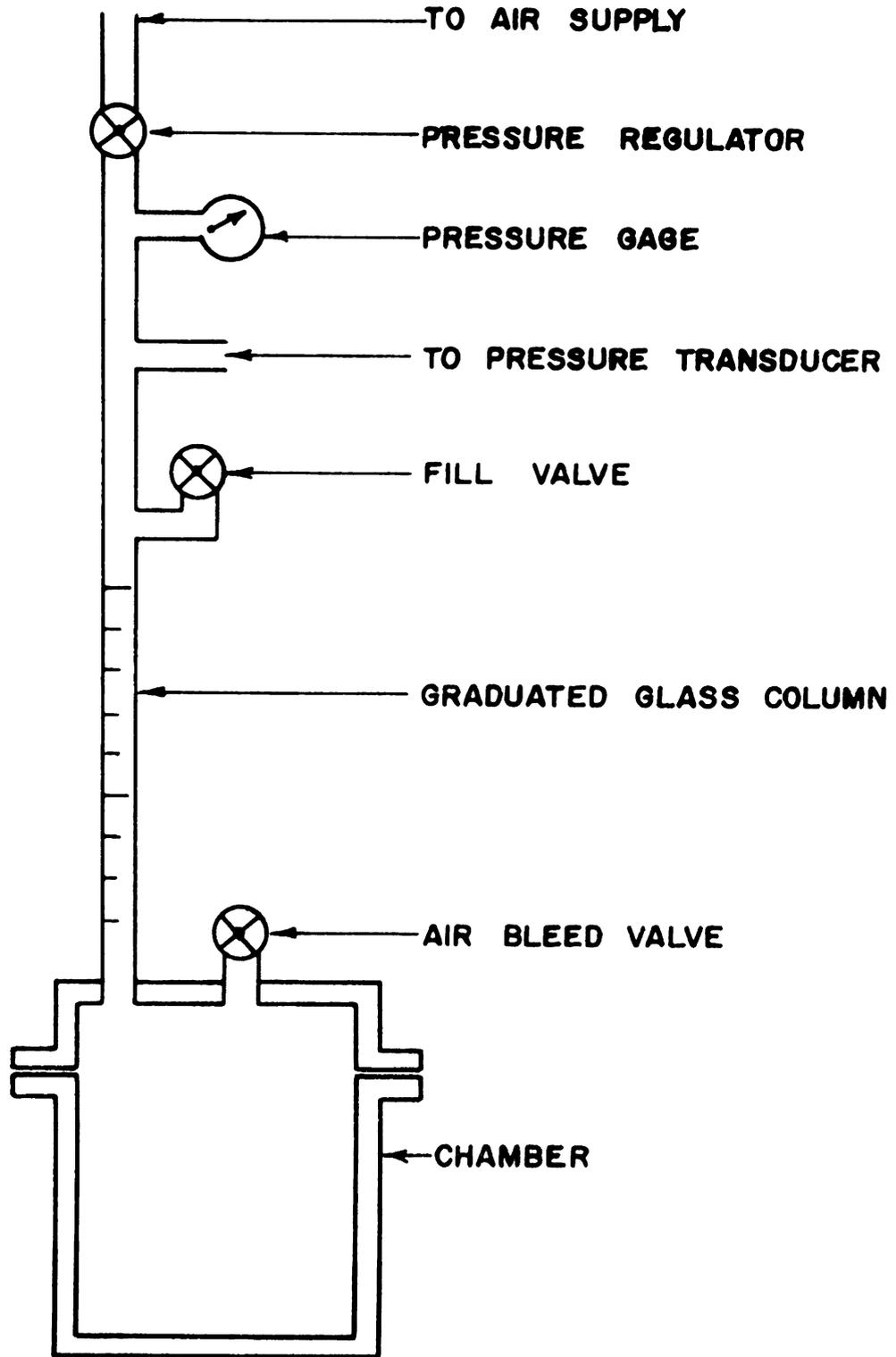
Figure 6.5.--Bulk Compression Apparatus.
