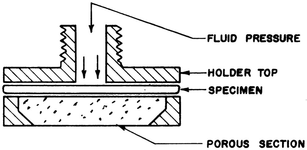
Figure 6.6.--Holder for Flat Specimen.
