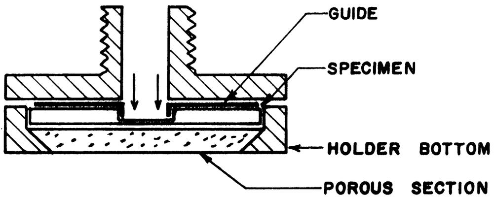
Figure 6.7.--Holder for Reduced Area Specimen.
