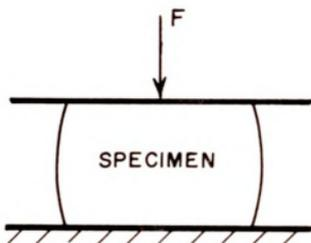
Figure 6.1.--Nonporous Flat Plate Loading.
