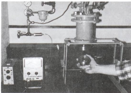
Figure 6.9.--Permeability Apparatus. Included are specimen holder, fluid supply, regulated pressure source, and pressure readout. (Photo 69-80)
