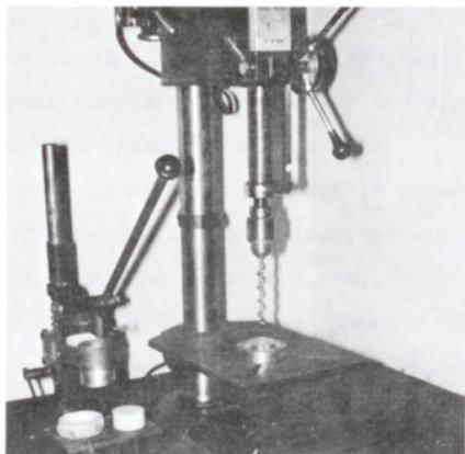
Figure 6.8.--Apparatus for Cutting of Reduced Area Permeability Specimen. Press on left was used for initial external cut. Press on right was used to cut center blind hole. (Photo 69-77)
