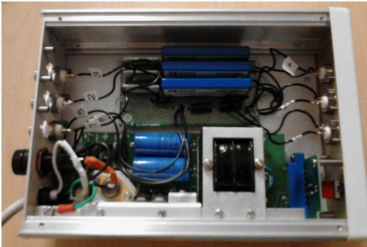
Figure 59. The voltage signal conditioning circuit.
