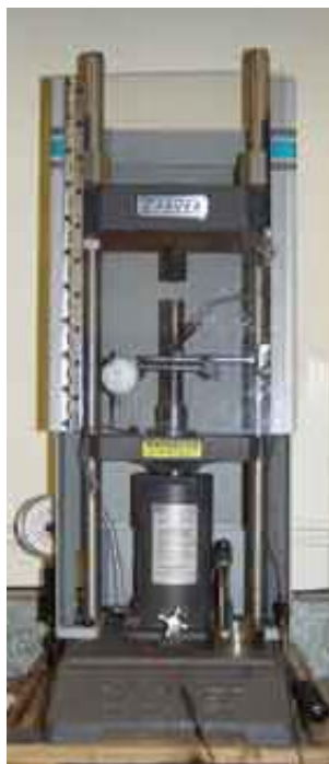
Figure 3.1: Uniaxial Press Device. Uniaxial press used to produce green strength electrolyte samples [115].
