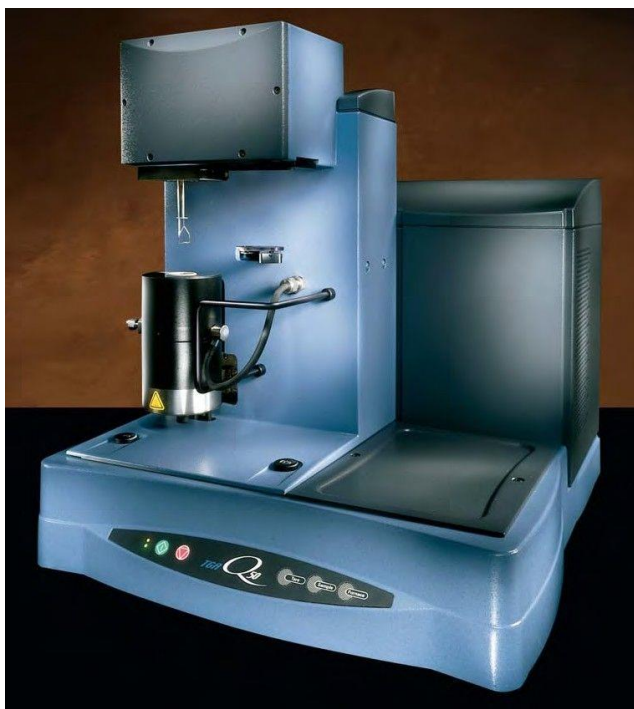
Figure 3.7: Thermo-Gravimetric Analysis Schematic. The depicted Thermo-Gravimetric Analysis uses a hanging scale to measure mass changes. [123].
